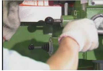
Step 2 Grasp the feeding lever using right hand and release the spindle to its utmost position.
