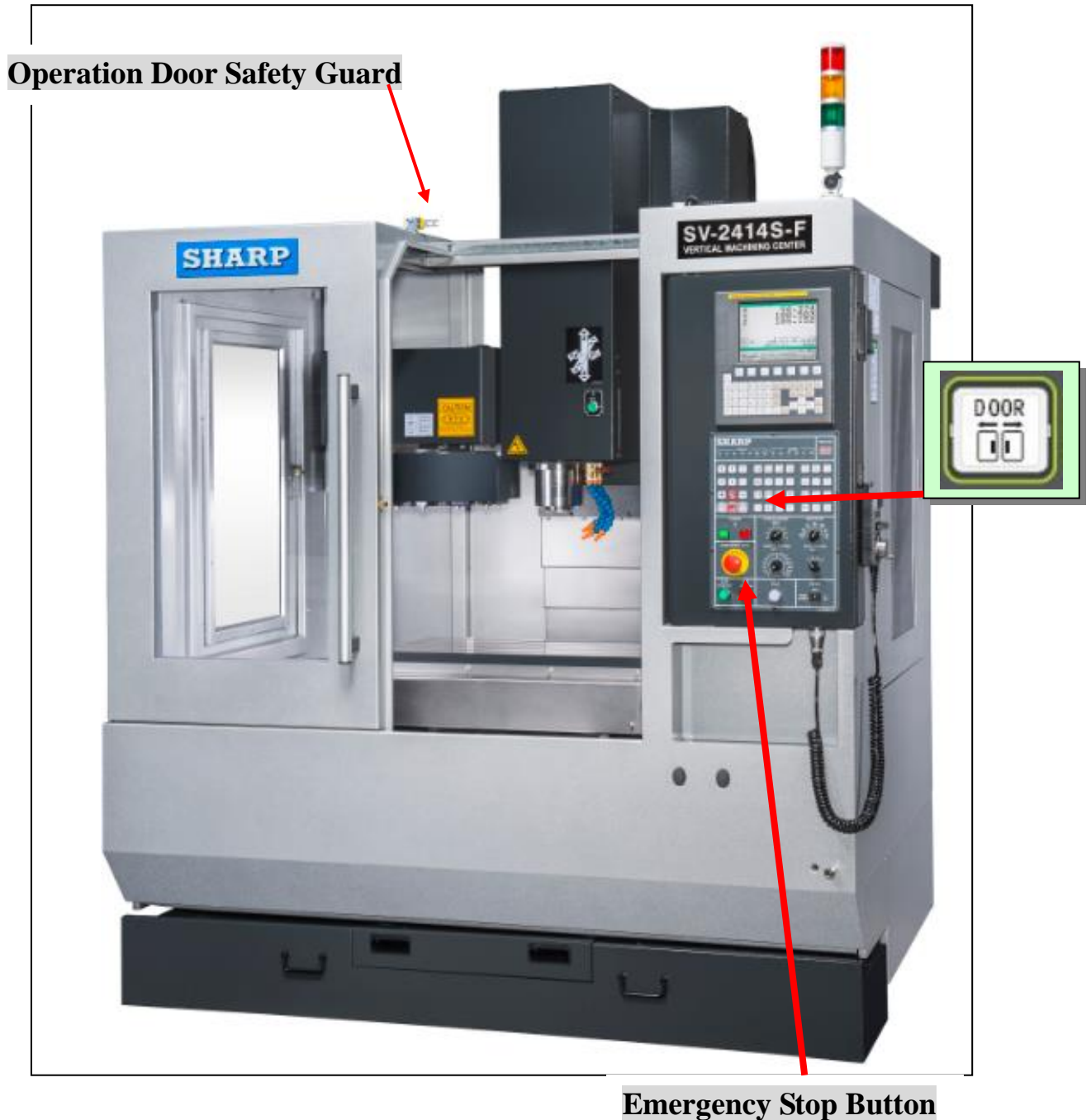
Figure 4.1 position of splashguard door and operation
