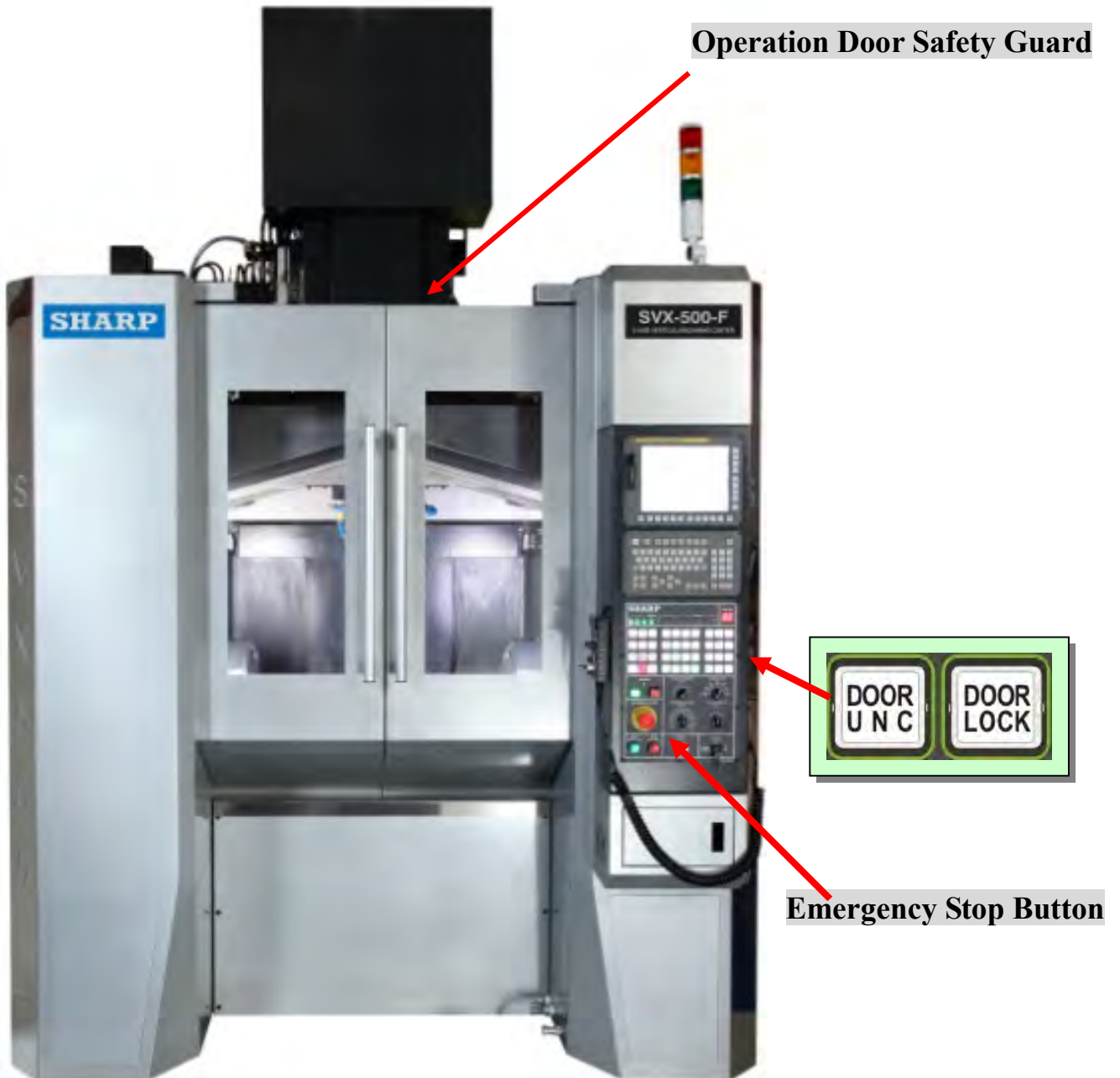
Figure 4.1 position of splashguard door and operation
